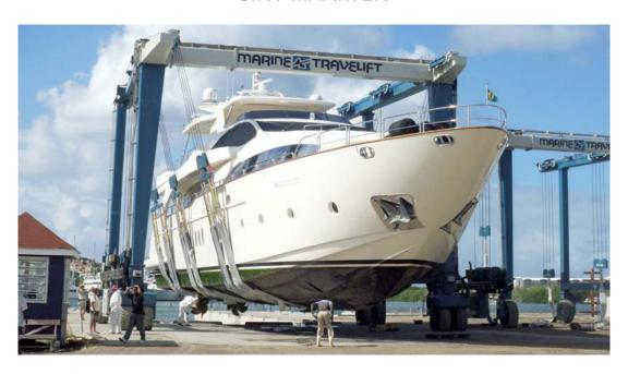
he Megayard in Sint Maarten has been open now for 5 years and is located in Cole Bay across the lagoon from Simpson Bay Yacht Club. This branch has 2 Travelifts: a 150 metric ton (165 US ton) machine that can haul vessels up to 33 feet wide. And a second machine of 75 tons for the smaller sail boats. This machine can accommodate a 19 foot wide vessel.
