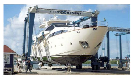
he Megayard in Sint Maarten has been open now for 10 years and is located in Cole Bay across the lagoon from Simpson Bay Yacht Club. This branch has 2 Travelifts: a 150 metric ton (165 US ton) machine that can haul vessels up to 33 feet wide. And a second machine of 75 tons for the smaller sail boats. This machine can accommodate a 19 foot wide vessel.
