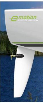
rudder bearing to handle the thrust) that the prop came out of the water during severe pitching. Another problem: With a scoop transom and swimmers, this puts feet and prop in too close proximity. (Even sitting on the transom with feet or hands in the water was a danger on some early models.)
