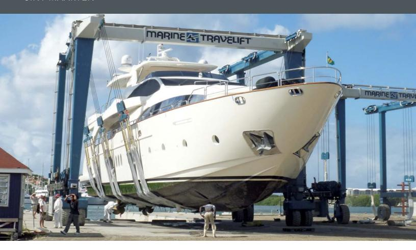
he Megayard in Sint Maarten has been open now for 10 years and is located in Cole Bay across the lagoon from Simpson Bay Yacht Club. This branch has 2 Travelifts: a 150 metric ton (165 US ton) machine that can haul vessels up to 33 feet wide. And a second machine of 75 tons for the smaller sail boats. This machine can accommodate a 19 foot wide vessel.
