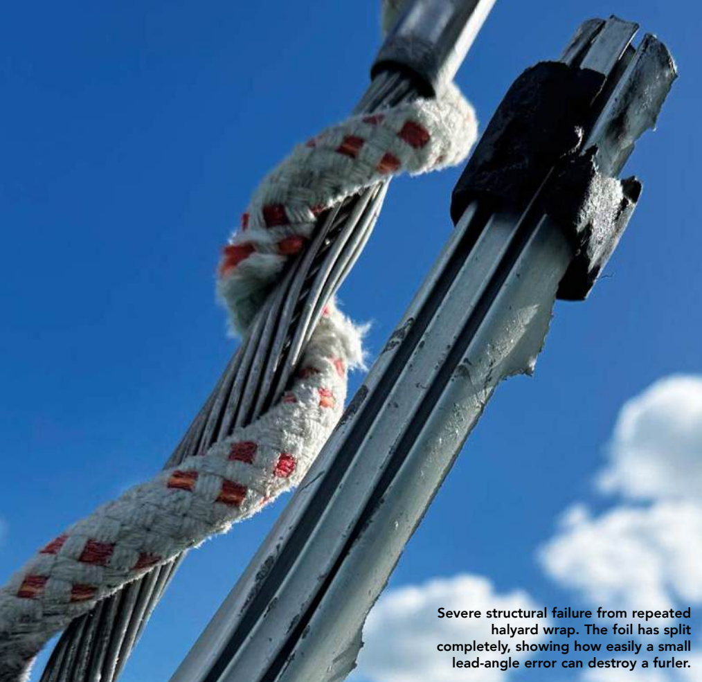
Another view of halyard wrap destruction. The extrusion has torn along its seam, the result of trying to keep furling instead of stopping to inspect.
