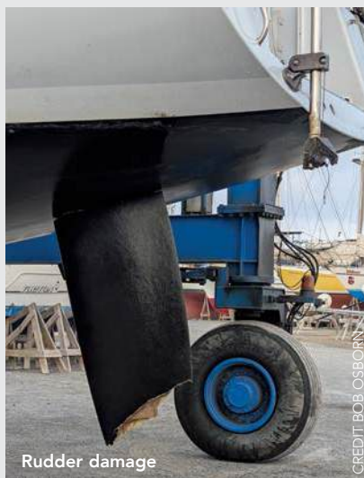
Holding SV Pandora's orca-broken rudder
